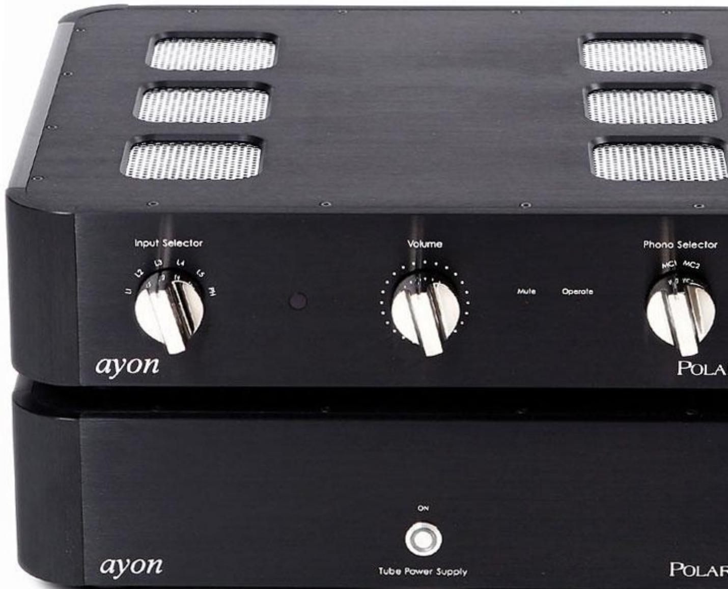
The Polaris is a two-chassis tube preamp design. One piece is the power supply and the other is the preamp. The components are of the exact same size, and while they are a bit on the large side, I was able to fit them into a four-shelf rack rather easily. Dimensions are 21x18x5 inches for each unit and they weigh in at 72.6 lbs for the pair.
